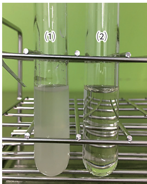
Figure 3. Maintenance of clarity of liquid dextrin (1): Control (dextrin) (2): Glyco Transferase-treated Both preparations were stored at 5°C for 5 days.
